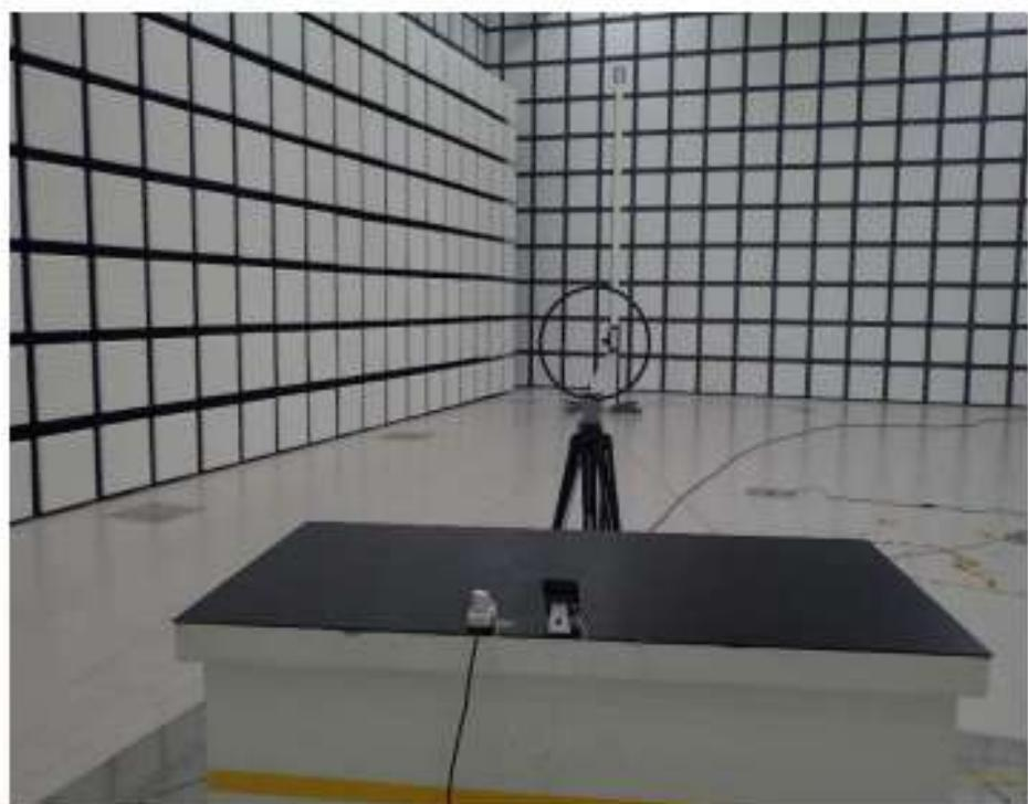
[ Test setup for above 30 MHz ]
