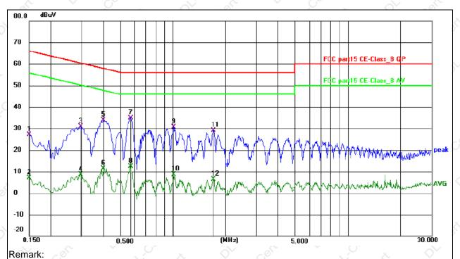
Margin = Level - Limit, Correct Factor = Cable lose + LISN insertion loss, Level= Reading + Correct factor
