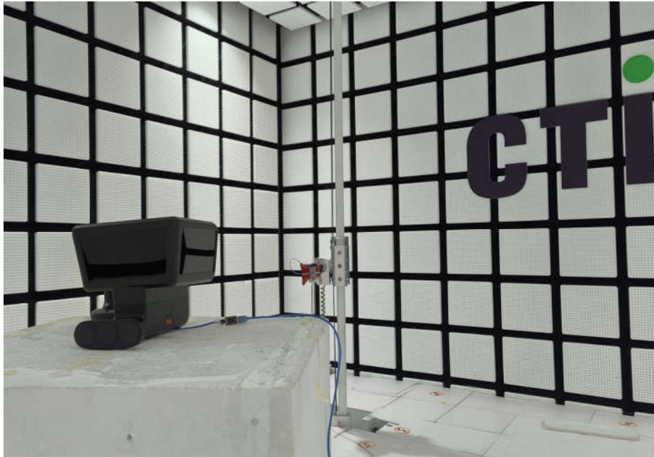
Radiated spurious emission Test Setup-4(Above 1GHz)
