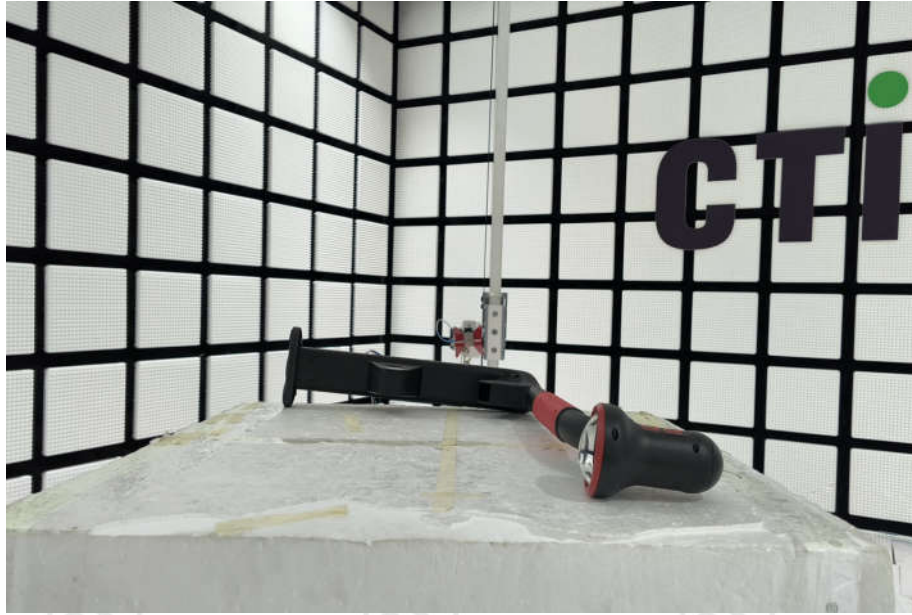
Radiated spurious emission Test Setup-3(Above 1GHz)
