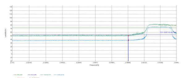
Suspected List Factor Limit Freq. Reading Level Margin [dB] NO Result **Polarity** Remark [MHz] [dBµV]  $[dB\mu V/m]$ [dBµV/m] [dB] 2390 13.75 36.91 50.66 74.00 23.34 **PASS** Vertical PΚ 1 2 2390 13.75 24.08 37.83 54.00 16.17 **PASS** Vertical ΑV
