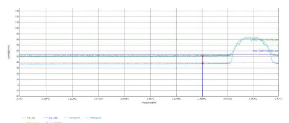
Suspected List Factor Limit Freq. Reading Level Margin [dB] NO Result **Polarity** Remark [MHz] [dBµV]  $[dB\mu V/m]$ [dBµV/m] [dB] 2390 13.75 37.25 51.00 74.00 23.00 **PASS** Vertical PΚ 1 2 2390 13.75 24.05 37.80 54.00 16.20 **PASS** Vertical ΑV
