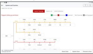
The system supports both topological graph and list display. Users can also click on "ADAS Calibration" to perform the vehicle's ADAS-related test options.
