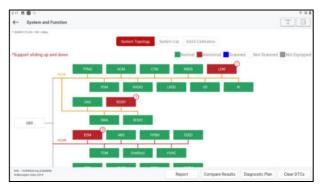
The systems with fault codes will be displayed on the screen with a red bottom box, and the number of specific fault codes will be displayed. Clicking on an individual system will allow the users to view the specific fault information. For systems without faults, the bottom box color is displayed in green.
