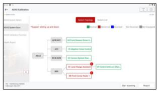
The ADAS system supports both topological graph and list displays. Click **Start Scan** to start scanning ADAS systems one by one. After the scanning is completed, click on the system that is displayed in red (the system is displayed in red, which means that there is a fault code for the system) to view the fault code, and click on the system that is working normally (the system is displayed in green, which means that the system is working normally) to perform other diagnostic functions
