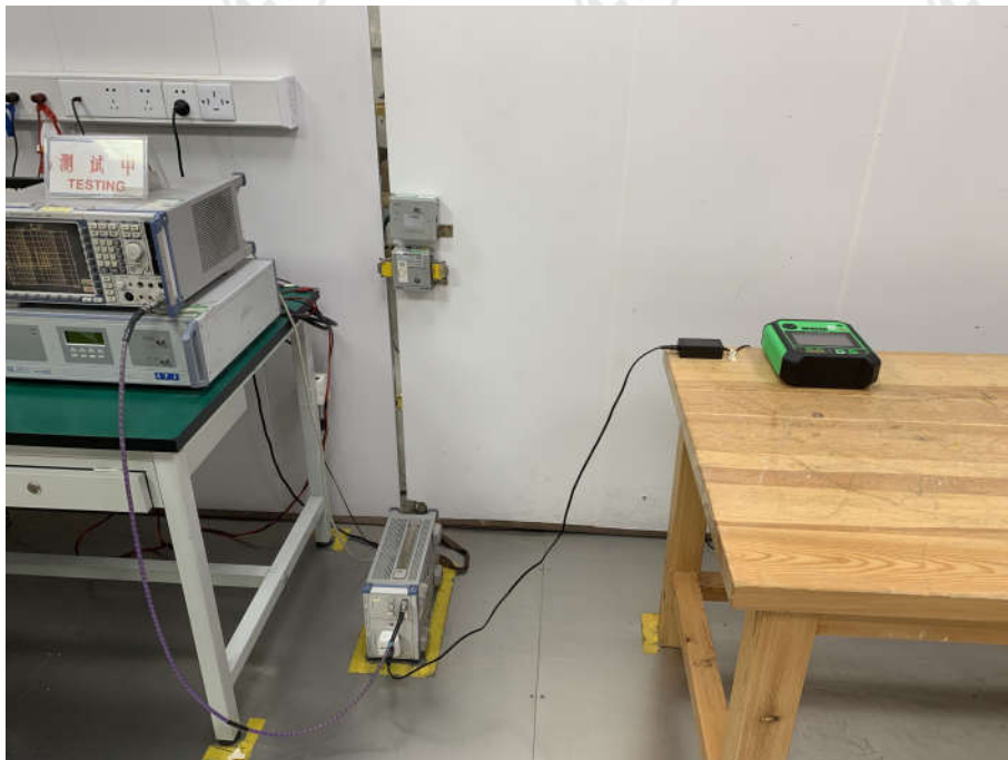
Conducted Emissions Test Setup
