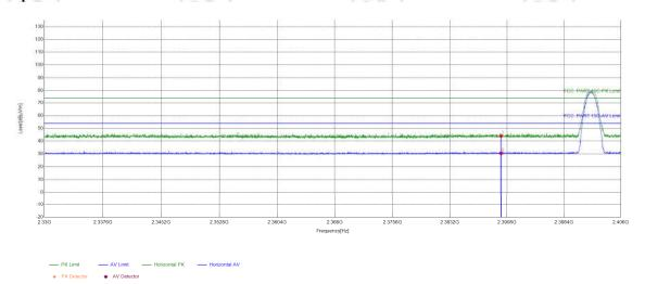
**Suspected List** Factor Limit Reading Level Margin Freq. [dB] NO Result **Polarity** Remark [MHz] [dBµV] [dBµV/m]  $[dB\mu V/m]$ [dB] 1 2390 5.77 38.35 44.12 74.00 29.88 **PASS** Horizontal PΚ 2 2390 5.77 24.76 30.53 54.00 23.47 **PASS** Horizontal ΑV
