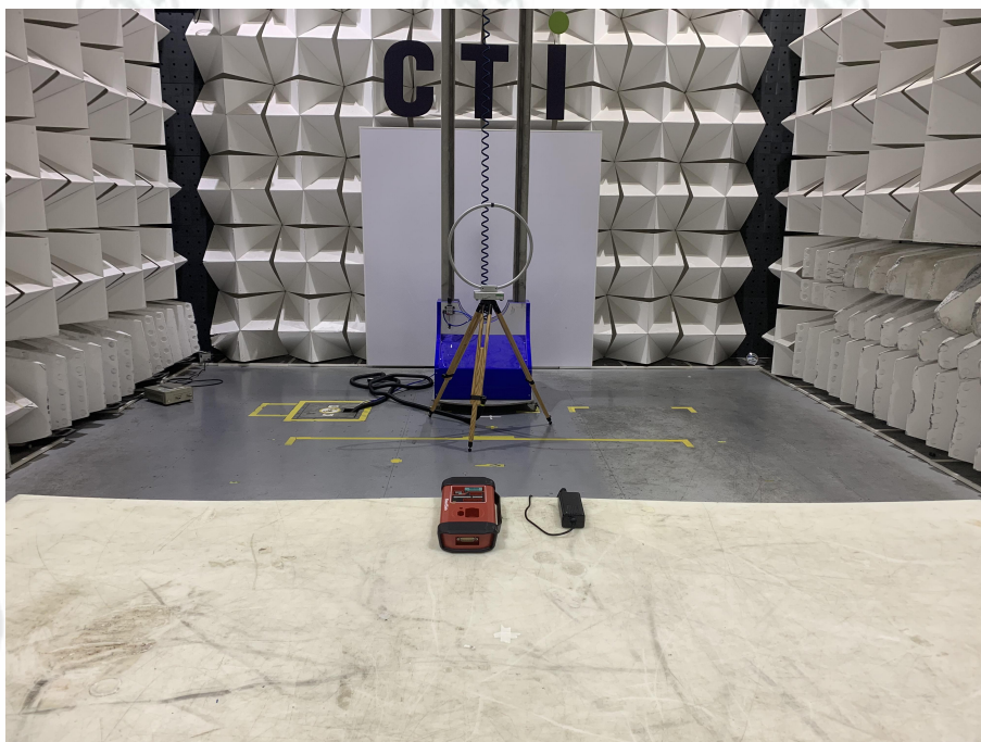
Radiated emission Test Setup (Below 30MHz)
