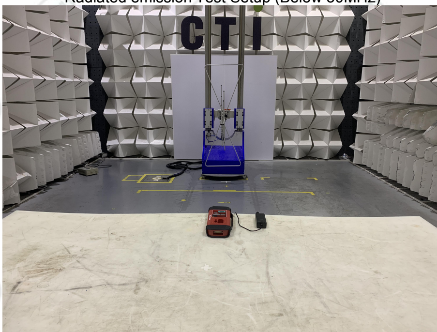
Radiated emission Test Setup (Below 1G)
