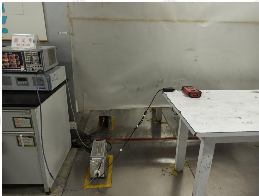
Conducted Emissions Test Setup
