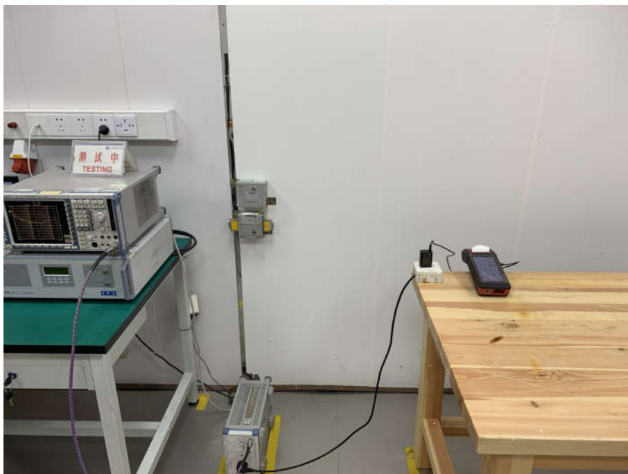
Conducted Emissions Test Setup
