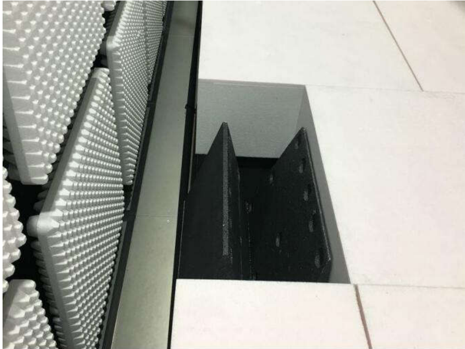
Radiated spurious emission Test Setup-4 There are absorbing materials under the ground.
