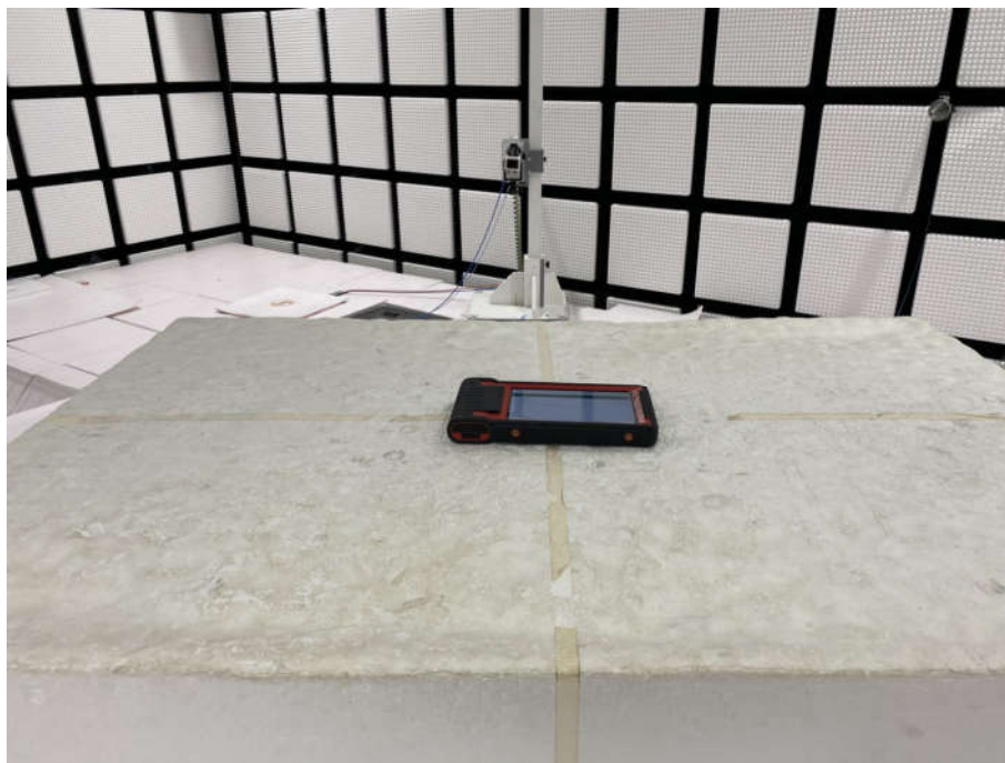
Radiated spurious emission Test Setup-3(18-30 GHz)
