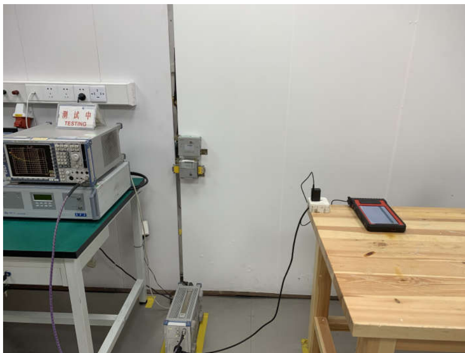
Conducted Emissions Test Setup
