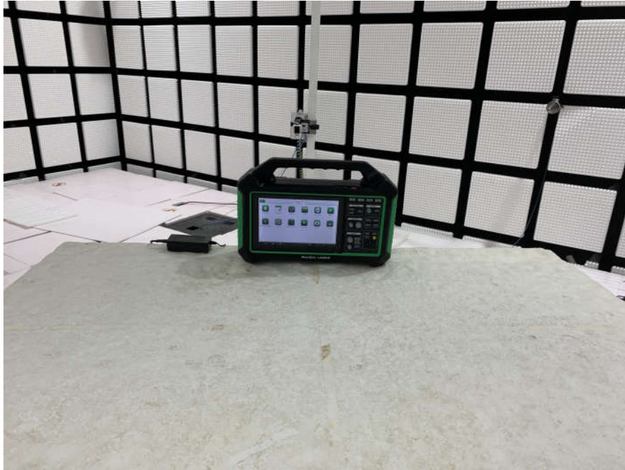
Radiated spurious emission Test Setup-3(Above 18GHz)
