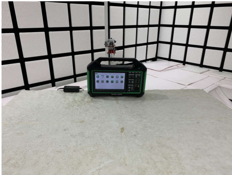
Radiated spurious emission Test Setup-2(Above 1GHz)
