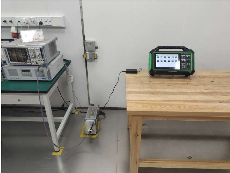
Conducted Emissions Test Setup
