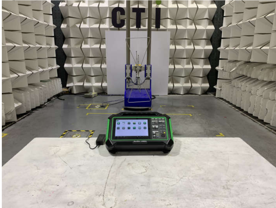
Radiated spurious emission Test Setup-1(Below 1GHz)
