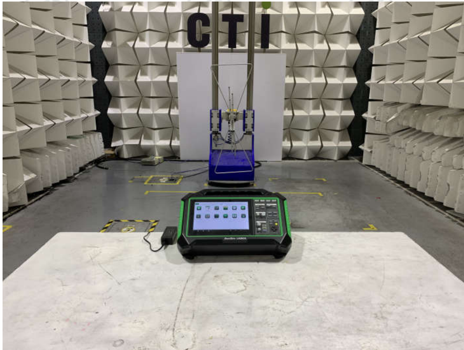
Radiated spurious emission Test Setup-1(Below 1GHz)
