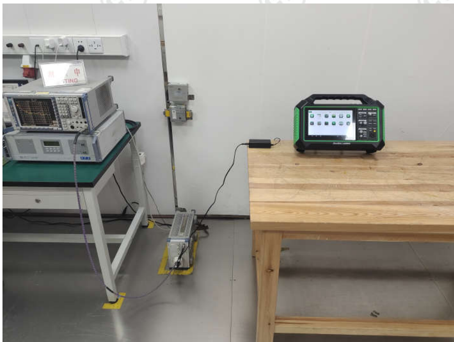
Conducted Emissions Test Setup
