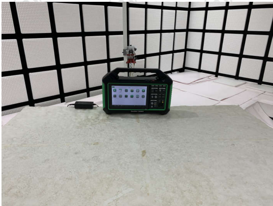
Radiated spurious emission Test Setup-2(Above 1GHz)
