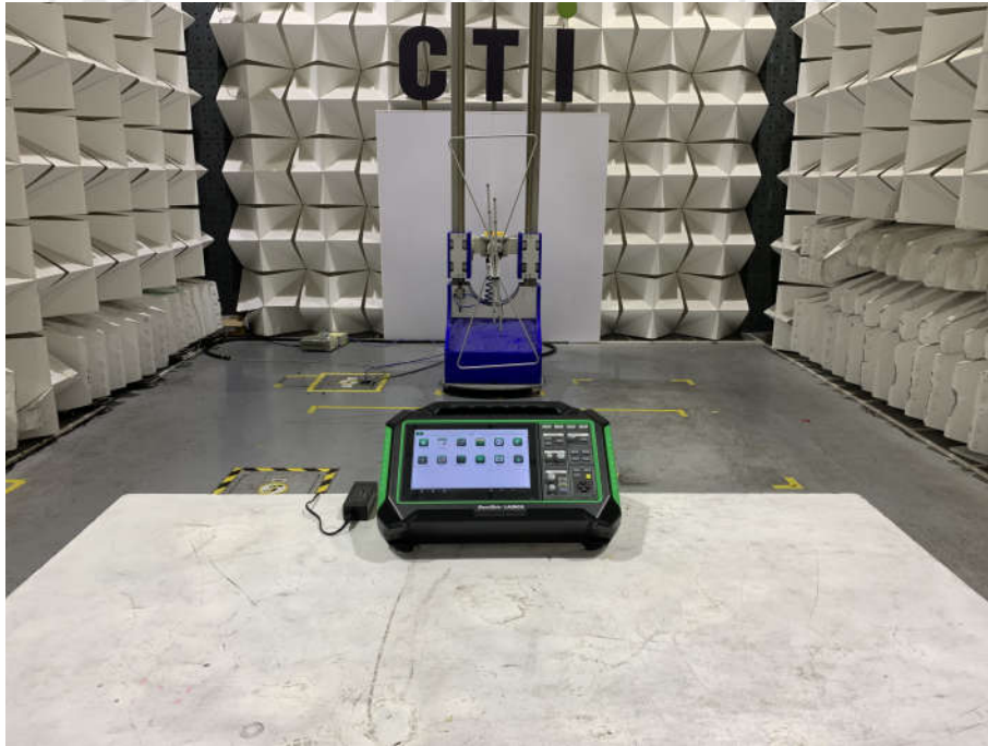
Radiated spurious emission Test Setup-1(Below 1GHz)
