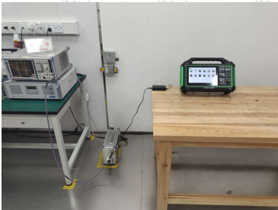
Conducted Emissions Test Setup
