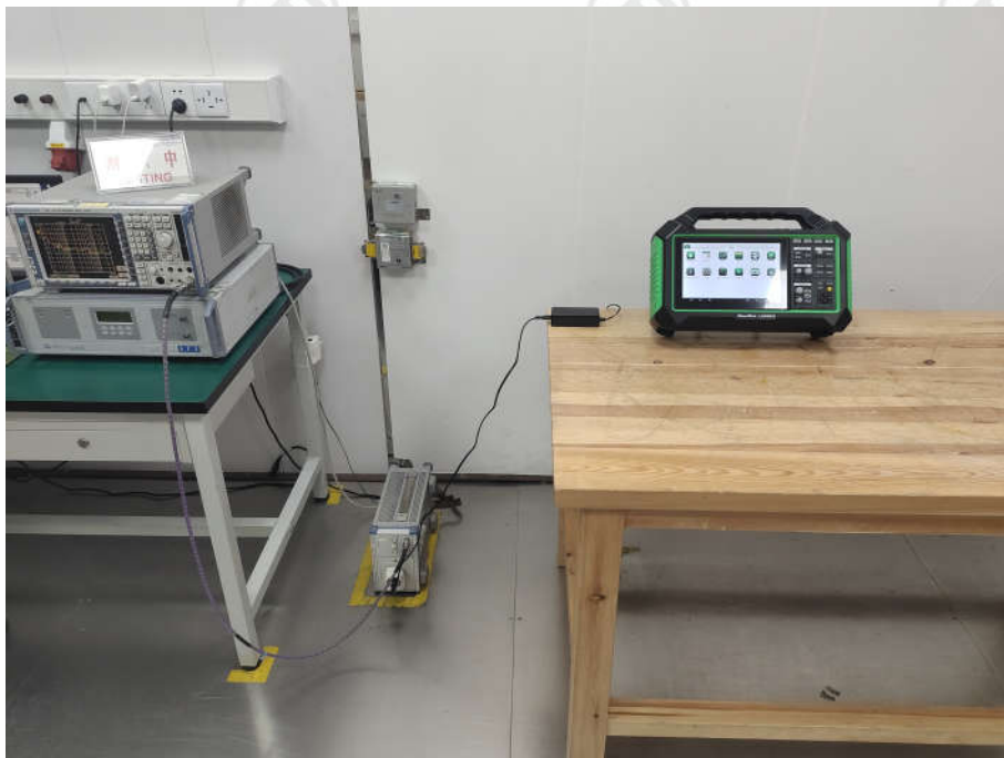
Conducted Emissions Test Setup
