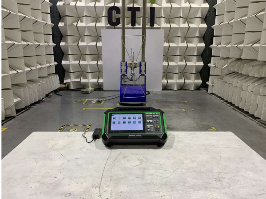
Radiated spurious emission Test Setup-1(Below 1GHz)
