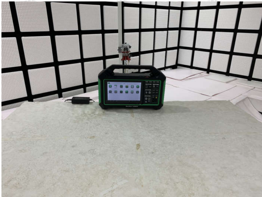
Radiated spurious emission Test Setup-2(Above 1GHz)
