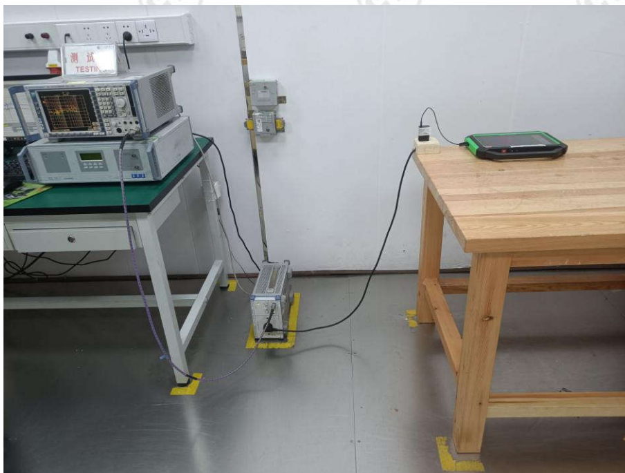
Conducted Emissions Test Setup
