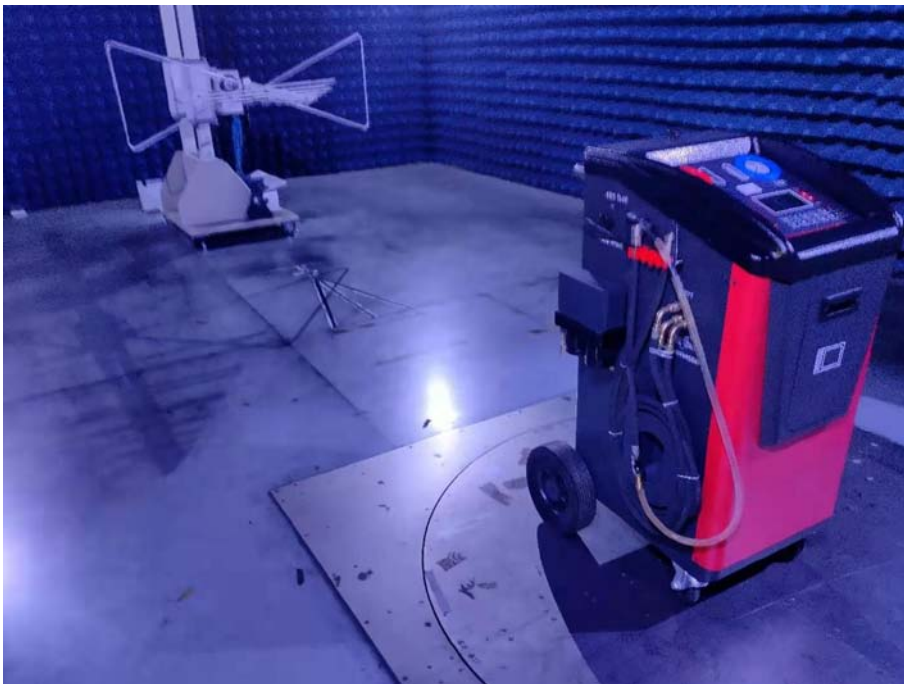
Photo of Radiated Emission Measurement Below 1GHz
