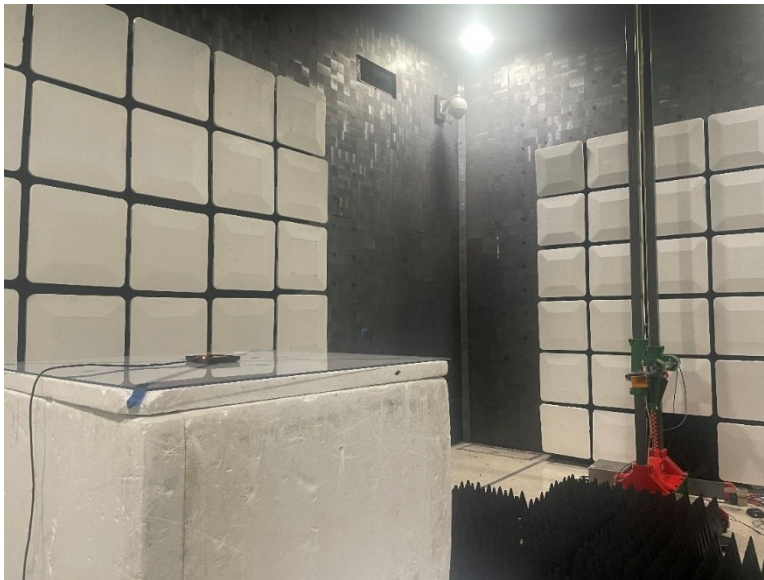
Figure 1.2-3: Radiated emissions setup (18 – 26.5 GHz): Front view photo.
