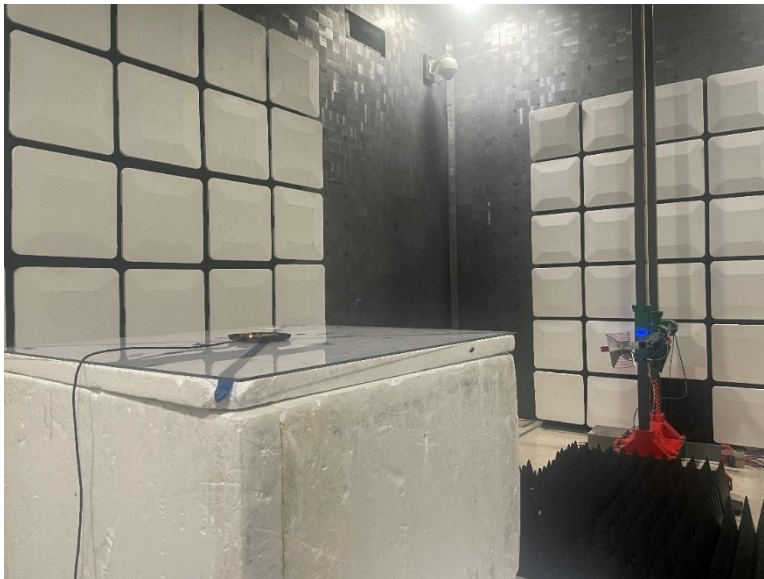
Figure 1.2-2: Radiated emissions setup (1 - 18 GHz): Rear view photo.
