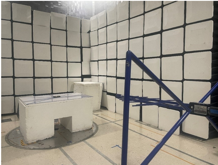
Figure 1.1-1: Radiated emissions setup (0.030 – 1 GHz): Front view photo.
