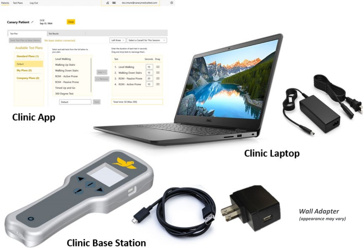
Figure 3: Clinic Base Station System Components
