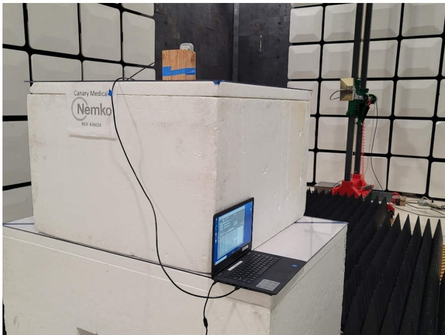
Figure 9- EIRP Measurement setup, rear view.
