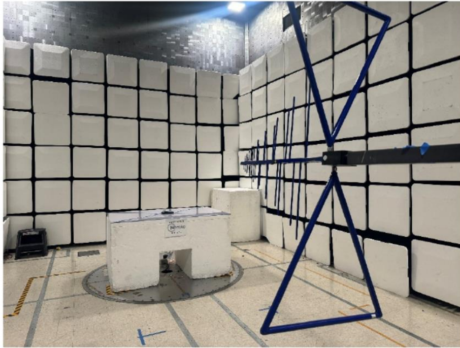
Figure 9.1-1: Radiated emissions setup (0.030 – 1 GHz): Front view photo.
