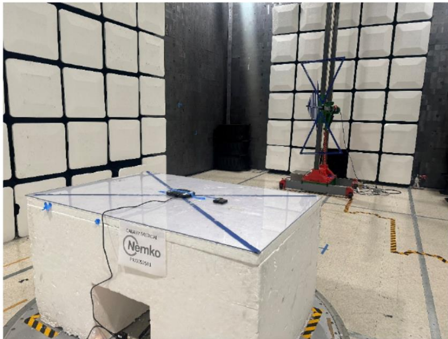
Figure 9.1-2: Radiated emissions setup (0.030 – 1 GHz): Rear view photo.
