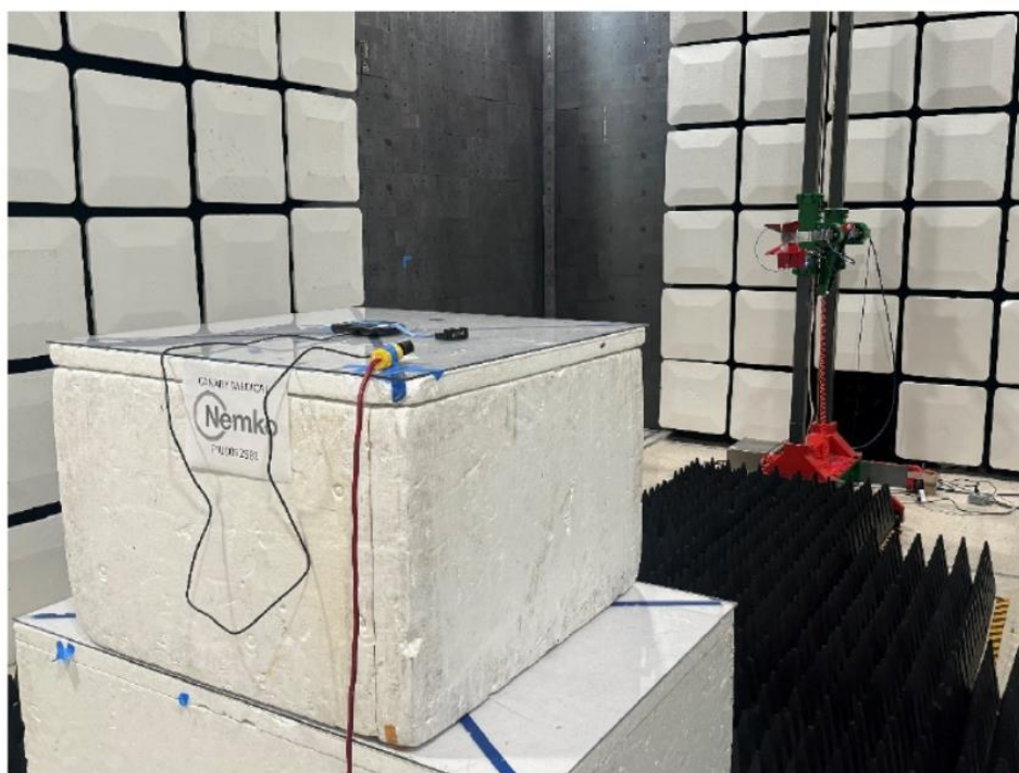
Figure 9.1-3: Radiated emissions setup (1 - 5 GHz): Rear view photo.
