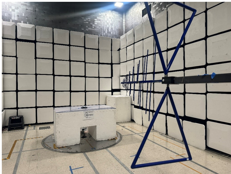
Figure 9.1-1: Radiated emissions setup (0.030 – 1 GHz): Front view photo.
