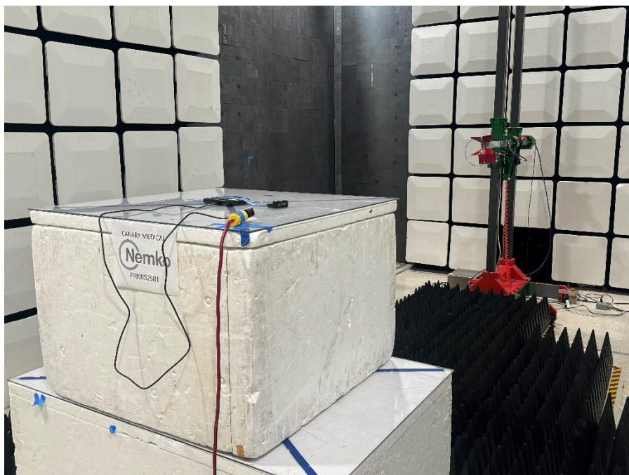
Figure 9.1-3: Radiated emissions setup (1 - 5 GHz): Rear view photo.
