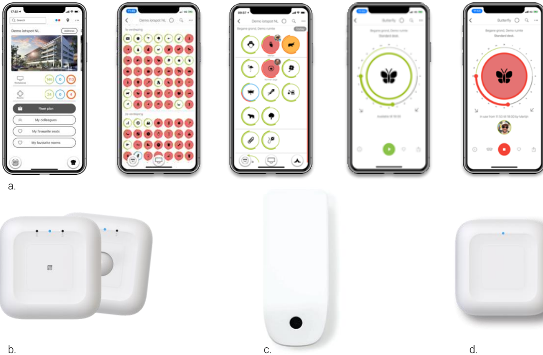
Figure 3. Ancillary products. 3.a An impression of smartphone app (iOS version) where you see the 1:1 relationship between the icon of the iotspot and its representation in the App by the same icon. 3.b The PIR-based desk and room (in the back) sensor that assess availability/occupancy based on motion detection. 3.c The camera-based sensor to assess the actual count of people in an area/room. 3.d The climate sensor that monitors the interior climate.
