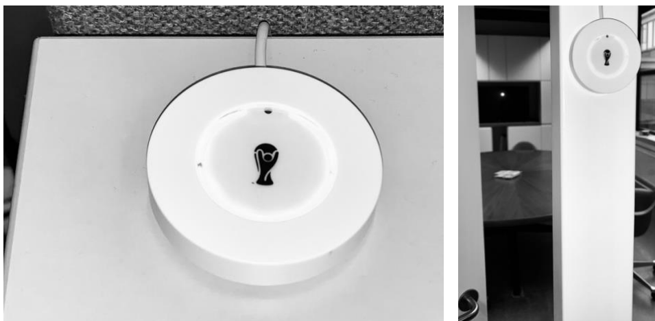
Figure 4. Position the iotspot at a top end corner of desk (left) or at eye level at the entrance of a meeting room (right).
