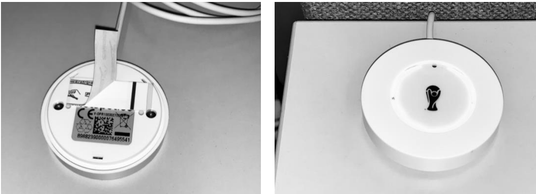
Figure 5. Mounting an iotspot on a desk without applying any mounting device. Fit and/or uncover the double-sided tape at the bottom side of the iotspot to stick the iotspot at its designated position.
