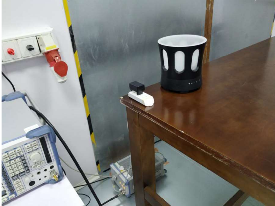
Conducted Emissions at AC Power Line (150kHz-30MHz)
