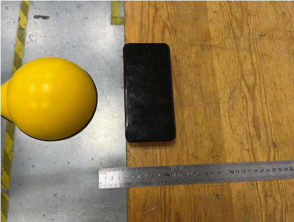
Test Position B(4cm) - Exposure photo from side edge surface-Rear(TM1)
