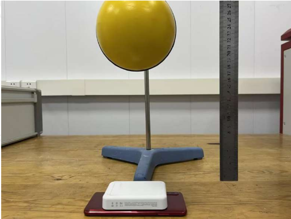
Test Position F(18cm) - Exposure photo from bottom surface(TM1)
