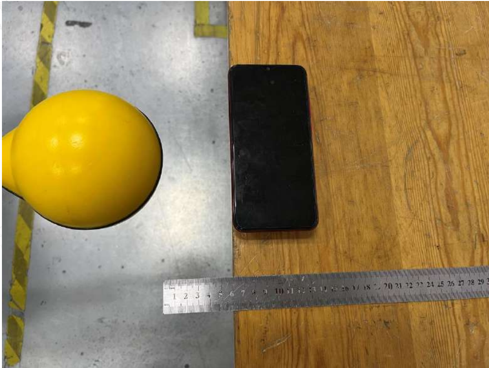
Test Position B(6cm) - Exposure photo from side edge surface-Rear(TM1)
