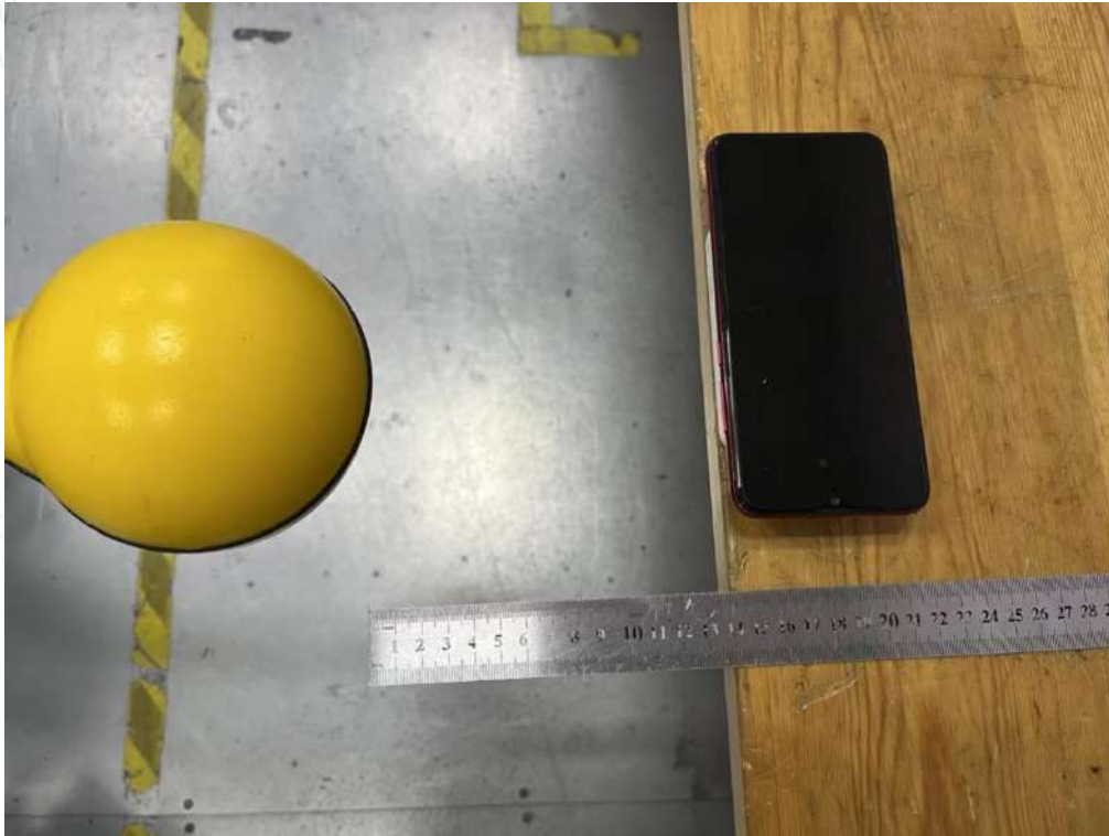
Test Position D(14cm) - Exposure photo from side edge surface-Front(TM1)
