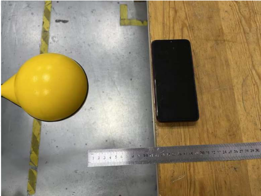
Test Position B(12cm) - Exposure photo from side edge surface-Rear(TM1)
