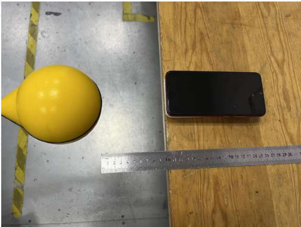
Test Position E(10cm) - Exposure photo from side edge surface-Right(TM1)
