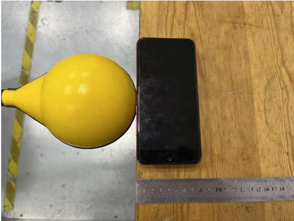
Test Position D(0cm) - Exposure photo from side edge surface-Front(TM1)
