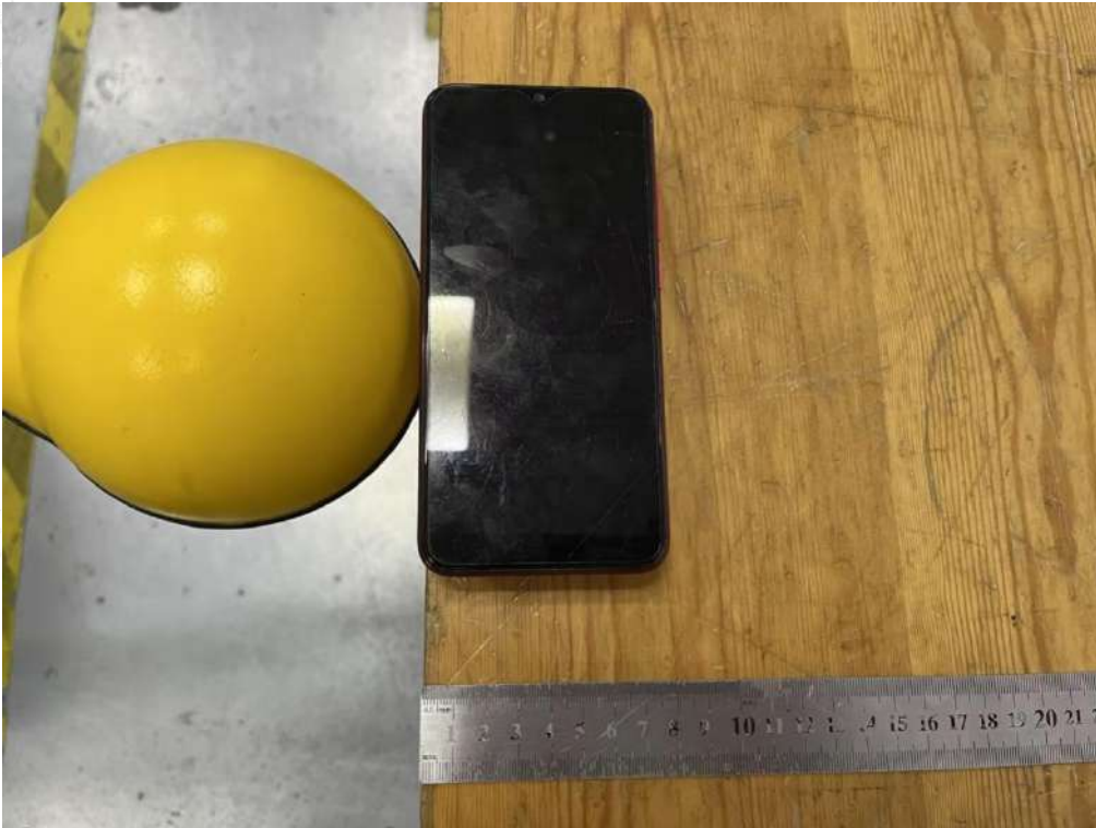
Test Position B(0cm) - Exposure photo from side edge surface-Rear(TM1)
