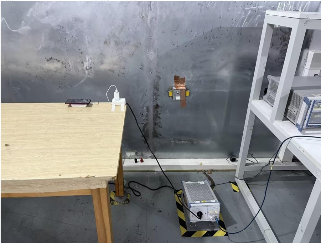
Conducted Emission-AC adapter charge mode
