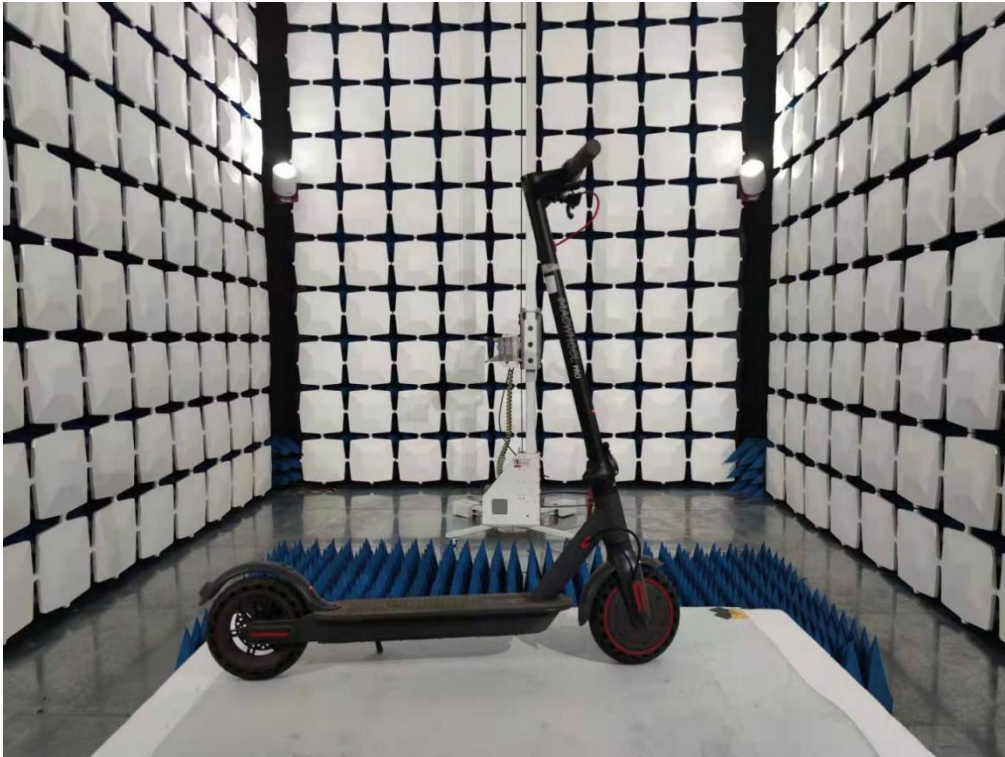
Below 1GHz for radiated emission test setup
