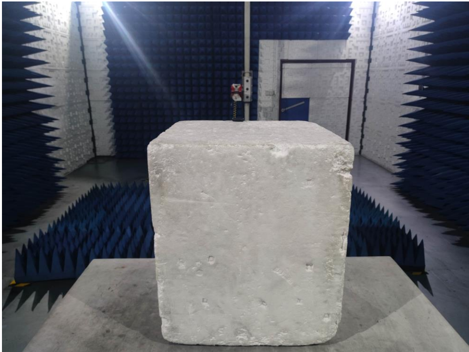
RADIATED EMISSION TEST SETUP ABOVE 1GHZ
