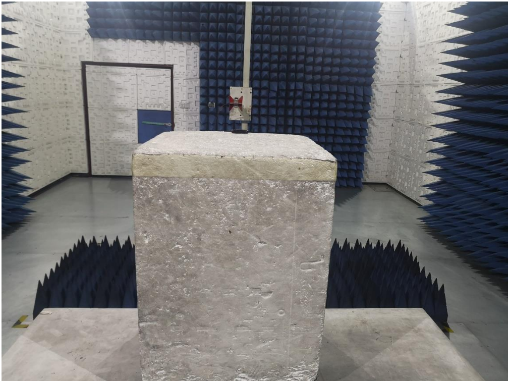
FCC RADIATED EMISSION TEST SETUP-ABOVE 1GHz
