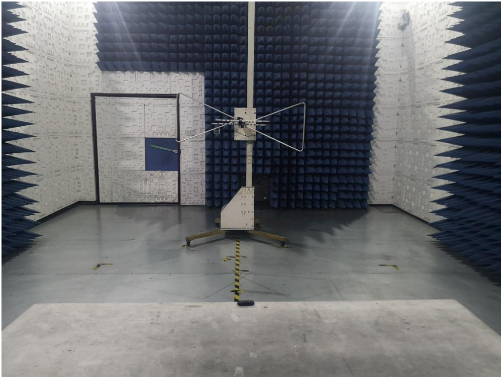
FCC RADIATED EMISSION TEST SETUP-ABOVE 1GHz
