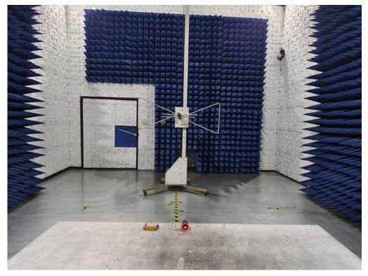
RADIATED EMISSION TEST SETUP ABOVE 1G
