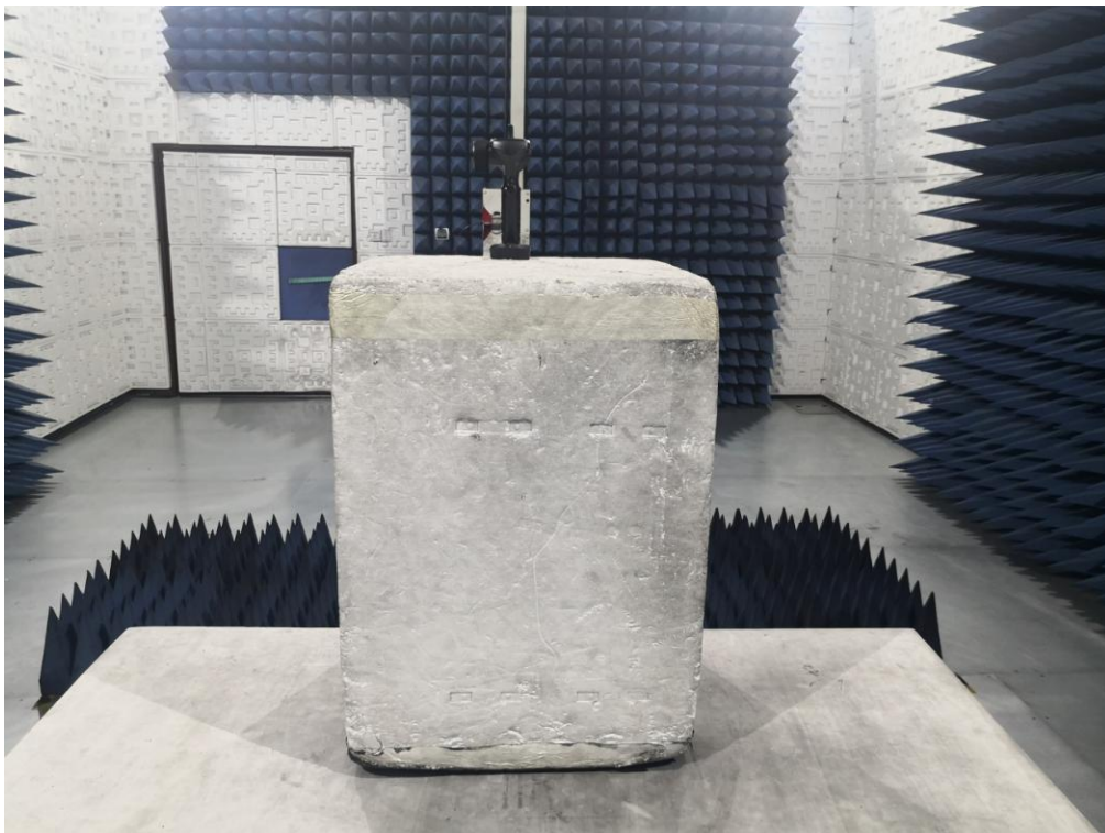
FCC RADIATED EMISSION TEST SETUP ABOVE 1GHZ
