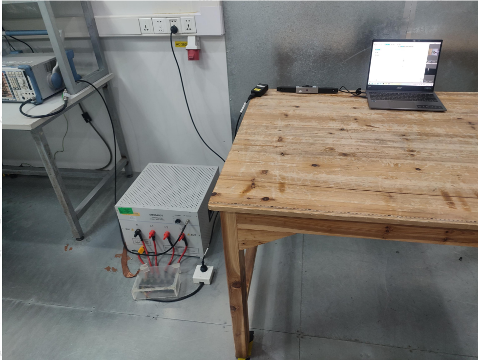
Photo of Conducted Emission Measurement
