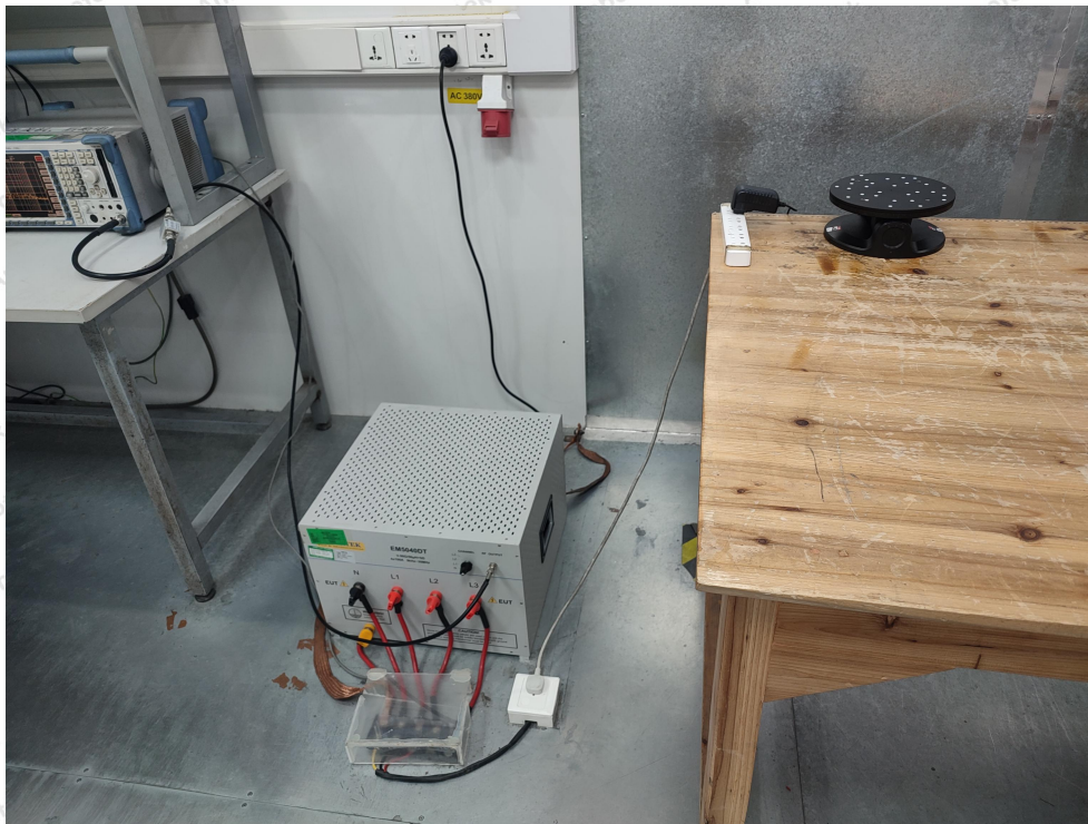
Photo of Conducted Emission Measurement
