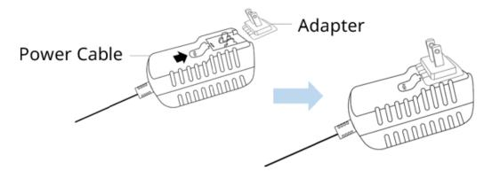
Step 2: Plug the Power Cable into a wall socket and the Dual-axis Turntable.
