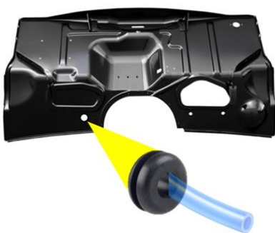
Figure 29: Air line Routed Through Firewall with Grommet
