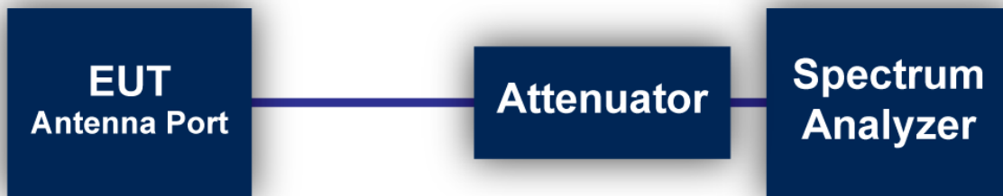
Figure 1: Direct Connection at the Antenna Port Test
