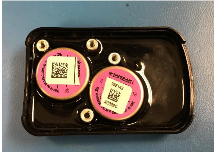
Photograph 3 – PCBA Potted in Housing View
