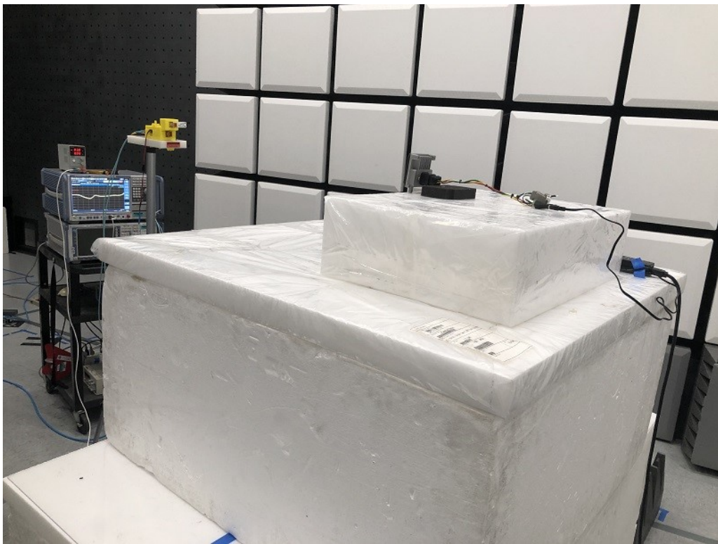
Radiated Emissions Test Setup (81GHz to 220 GHz)
