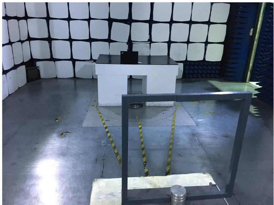
Radiation Emission Test Setup (Below 30MHz)
