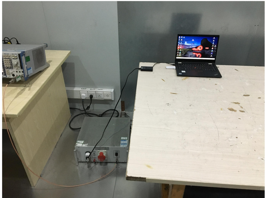
Conducted Emission Test Setup
