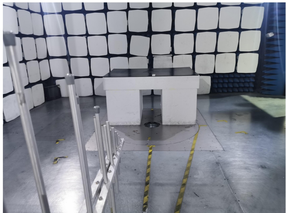
Radiation Emission Test Setup (30MHz to 1GHz)
