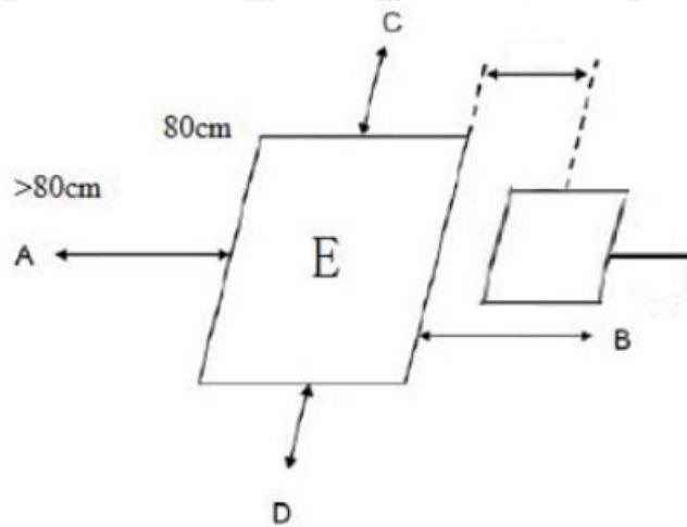
Note: Measurements should be made at 15 cm surrounding the EUT and 20cm above the top surface of the EUT. (probe radius is 4.75cm)
