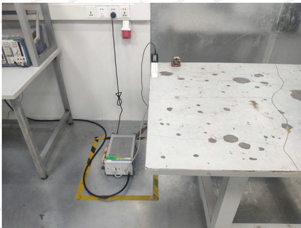
Photo of Conducted Emission Measurement
