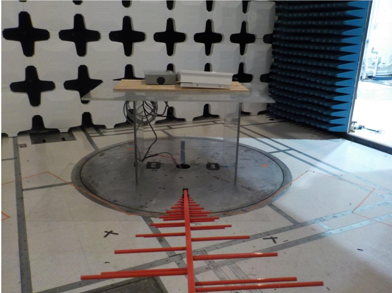
Figure 175: REE Setup (30Mhz-1Ghz)
