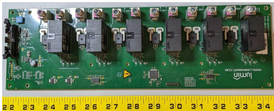
FRONT OF RELAY BOARD
