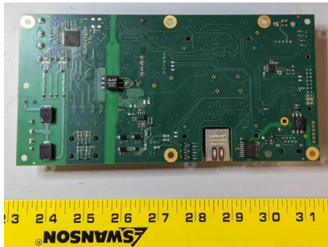
UNDERSIDE OF MAIN BOARD
