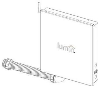
1 Outdoor LSP with Conduit, Conduit Bushings & Wire Whips Attached
