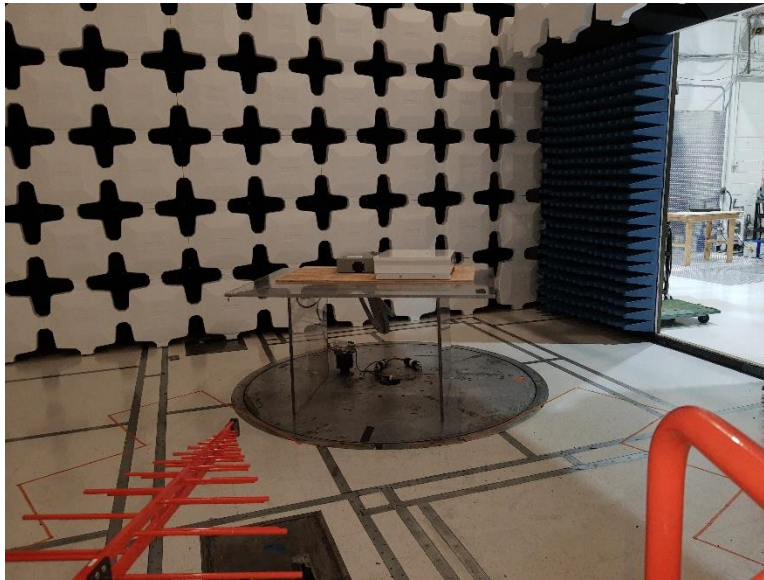
Photograph 2. REE Test Setup, 30-1000 MHz
