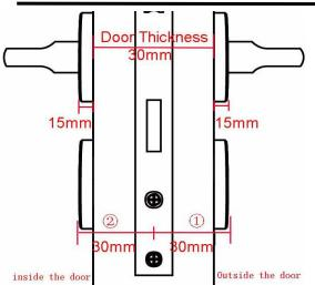
As shown in the figure: the door thickness is 30mm, and the panel thickness is 15mm, The distance of each compartment on the lock core is 5mm
