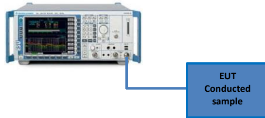
Figure 3.5-1: Test conducted setup.
