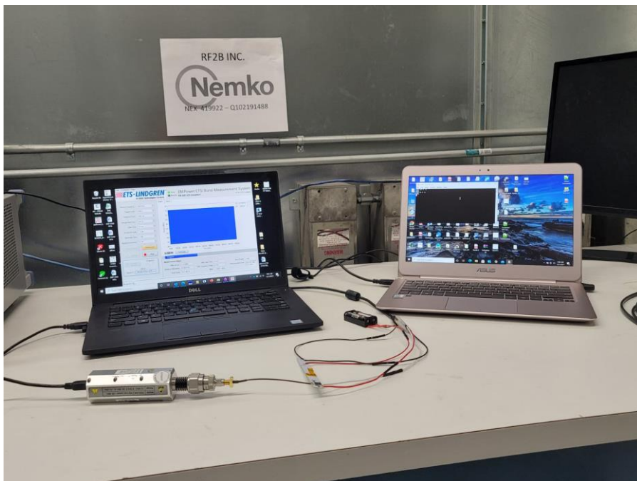
Figure 11 - Conducted emissions setup using a power sensor.
