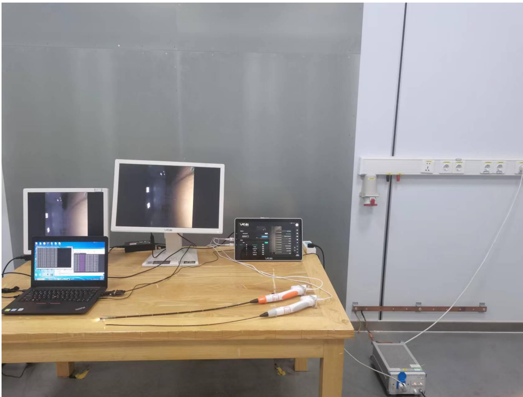
Fig. 4 Power line conducted emission setup photo
